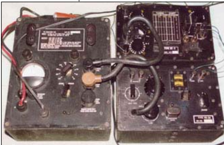
Figure 1. An RS-1 set, configured to operate from AC mains power. Clockwise from left are: power supply, RT-3 transmitter, and RR-2B receiver. The power supply shown will also operate from 6 VDC, and has a connector to receive input from a GN-58 hand-crank generator.
