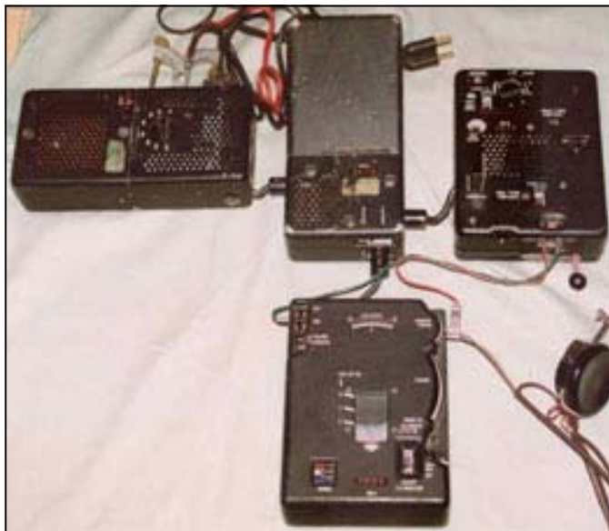
Figure 3. A complete RS-6 station ready for use from AC mains power. Clockwise from left: RP-6 power supply, RA-6 power filter unit, RT-6 transmitter, and RR-6 receiver. Note the tiny fold-out CW
