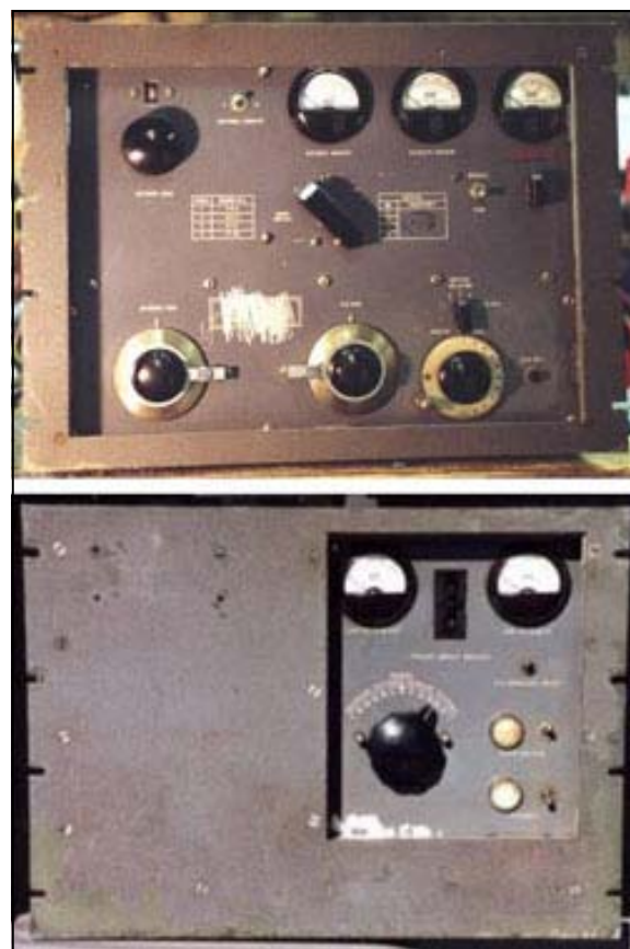
Figure 5. The RT-4 transmitter and power supply, which together weigh about 340 pounds. The identification has been thoroughly scratched off of the transmitter, to help hide its origin. The power supply's large variac knob is used to adjust for the input line voltage.
