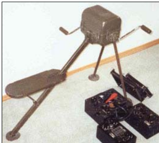
Figure 2. A GN-58 hand-crank generator, commonly used to power the RS-1 in the field.
