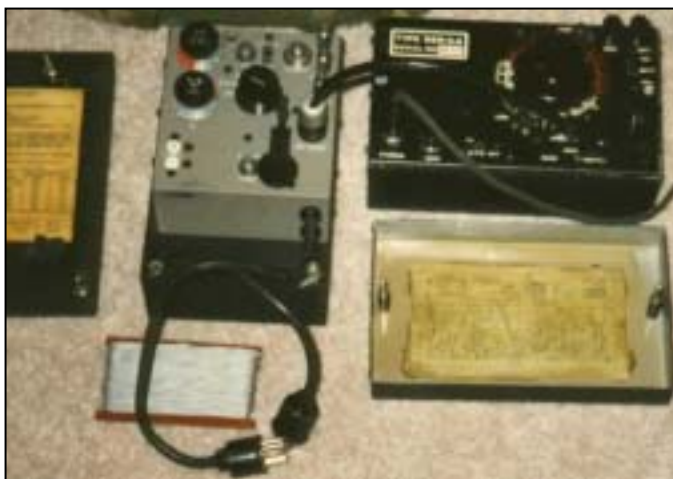
Figure 3. The transmitter and receiver of the SSTR-5 radio set. Image courtesy of Bill Howard.
