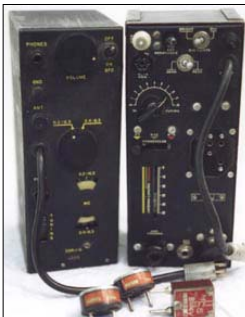
Figure 1. The SSTR-1's receiver and transmitter. The transmitter's crystal socket (on the right, center) accepts several different types of crystal holders. Image courtesy of Bill Strangfeld.
