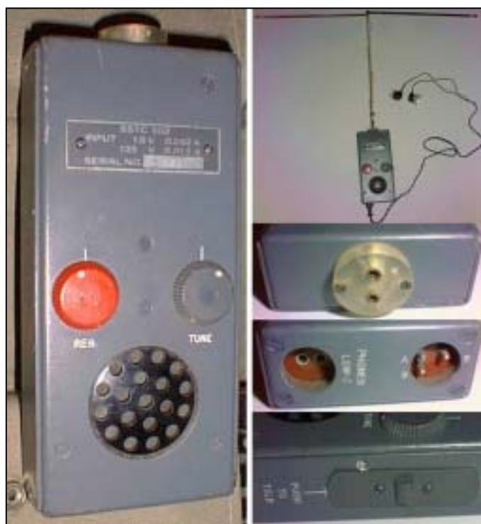
Figure 4. The handheld "Joan" (SSTC-502) portion of the Joan-Eleanor system. The upper-right image shows the folding antenna and earphones connected. Images courtesy of T.B.
