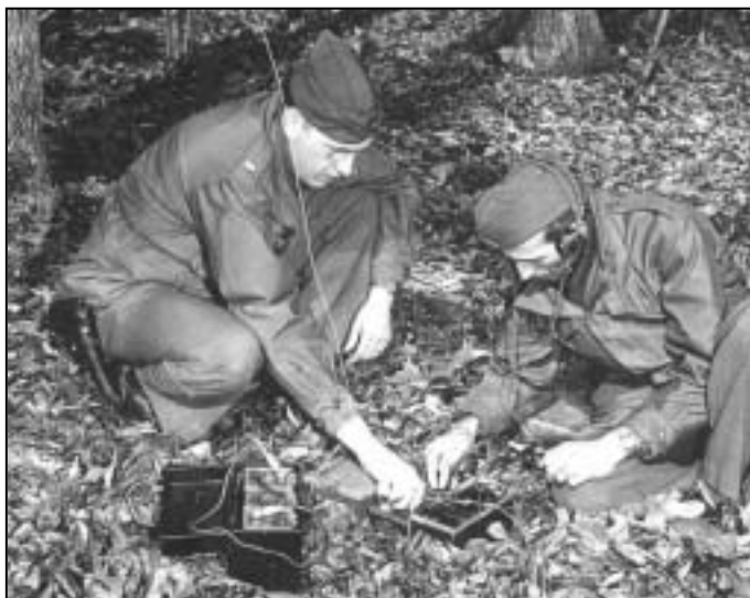
Figure 2. This picture shows an SSTR-1 set being operated from a 6V wet-cell battery, somewhere on the grounds of the OSS training base known as "Area C", in Virginia. National Archives photo.
