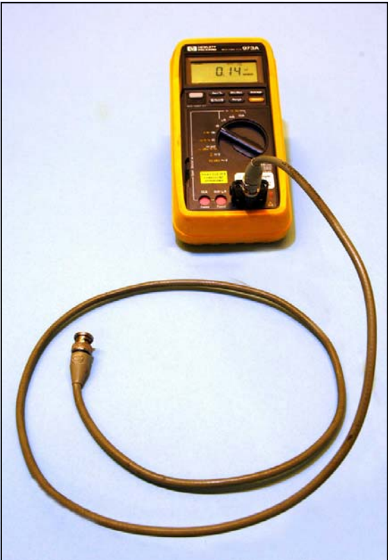
Measuring the capacitance of a known length cable.
