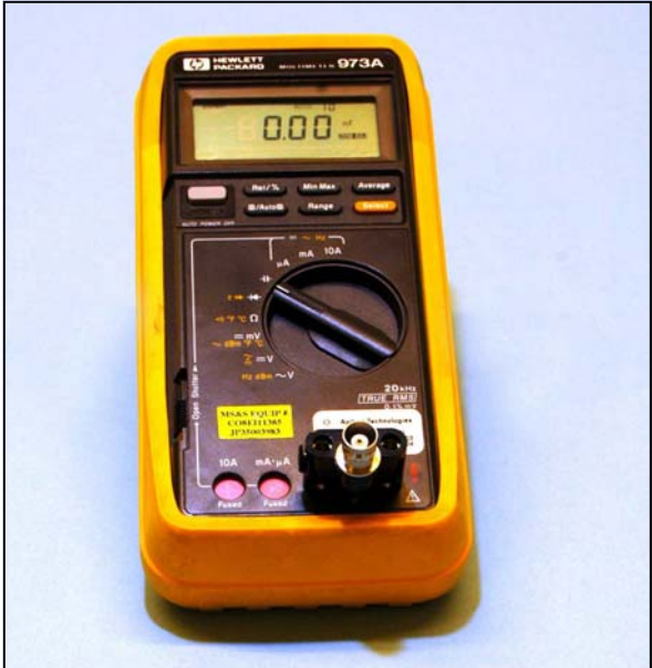
Zero the meter with coaxial adapter attached.
